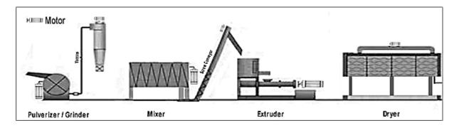
**Note:** Raw ingredients are poured into the pulverizer manually and the grained ingredients are transferred to the mixer chamber manually. After mixing, the ingredients will be poured into the extruder via a screw conveyor. Finally, the extruded feed will be transferred into the dryer chamber manually, where the moisture content is reduced and the feed is dried to the desired consistency.
